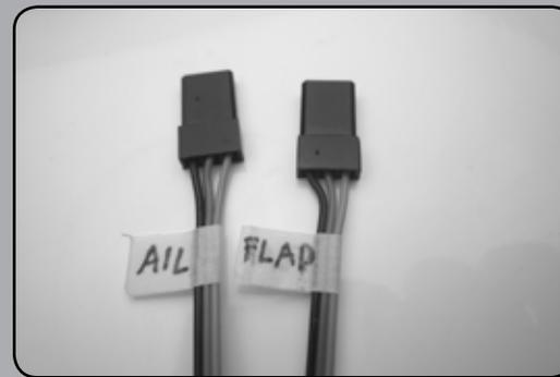
**Note:** Use your radio to center the flap servo before installing the servo hatch in the wing. The servo mounting location and pushrod length will position the flap with the trailing edge deflected 1/2-inch which is the mid-position. This measurement is made at the inboard end of the flap relative to the fixed portion of the wing trailing edge.
