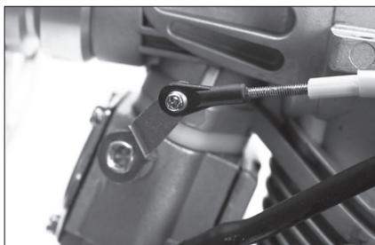
1. Use a secure method to attach the throttle linkage to the throttle arm on the carburetor.
