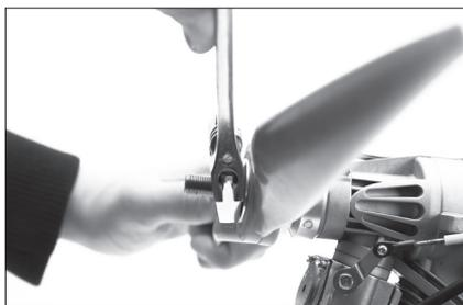
1. Remove the prop nut and prop washer from the crankshaft.
