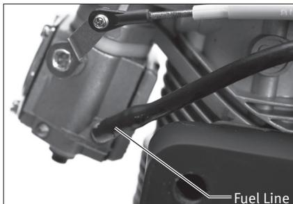
1. Connect medium diameter large diameter FKM fuel tubing to the carburetor and the fuel tank supply line.
