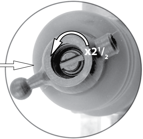
Low-Speed Needle - 2 1 / 2 turns out
