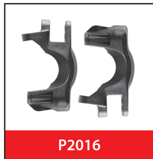
Caster blocks(c-hubs) C型座
